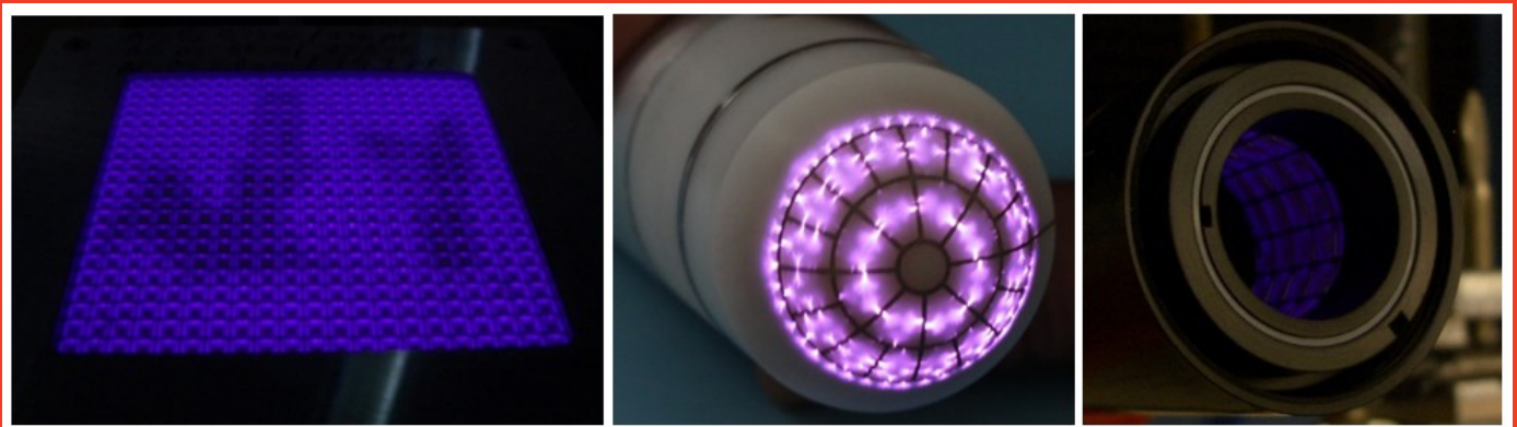
Figure 6: A selection of SMD cold plasma sources developed by terraplasma GmbH.
